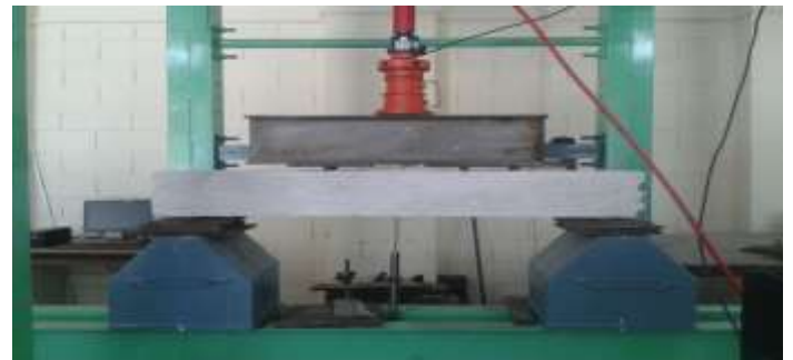
Figure 6.5: Test set up for flexural test of reinforced beams
