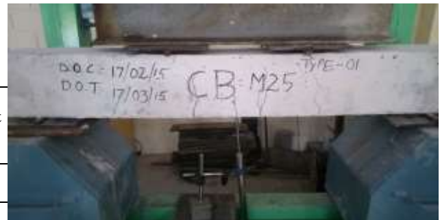
Figure 6.6: Crack pattern of control beam (Front face)
