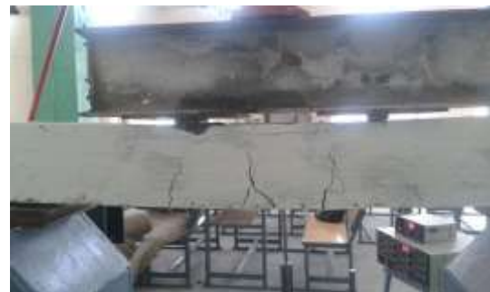
Figure 6.6: Crack pattern of control beam (Front face)
